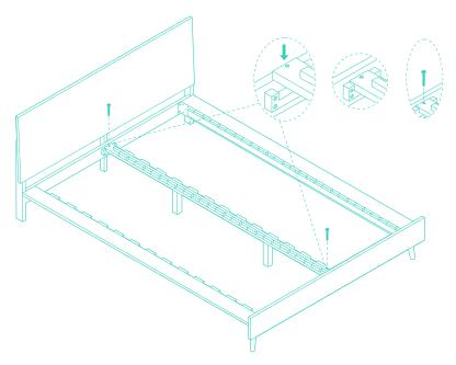
Drop the center support beam (I) into the existing U shaped supports on the headboard and footboard. Use two 32mm phillips screws (2) to secure the center beam on each end.
