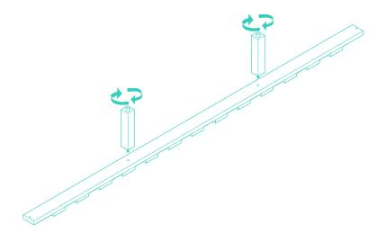
Attach the center support legs (**J**) to the center support beam (**I**) by threading the legs into the existing pilot holes on the center beam.
