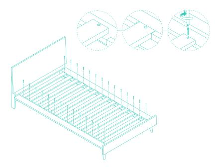
Drop one slat (**D**) into each of the matching slots on each side rail. Use a 32 mm phillips screw (**2**) to secure the slats to each side. Continue down the line. Tighten with a screwdriver.
