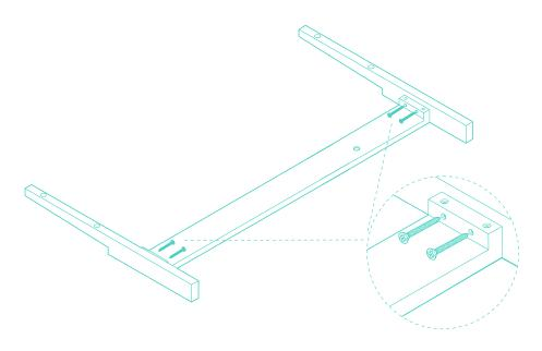
Attach the side headboard posts (**E**) to the headboard bar (**G**). Align the existing pilot holes of the side post to the holes of the headboard bar. Make sure the notch of the side post is facing the front of the support beam – as pictured. Thread two 32mm phillips screws (**2**) into the pilot holes to secure. Tighten with a screwdriver. Repeat on the other side.
