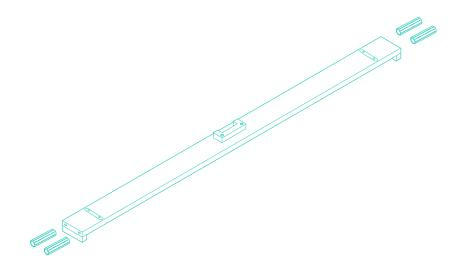
Find the existing pilot holes on the ends of each headboard bar (**G**). Place one wood dowel (**4**) into each hole as far as it will go.
