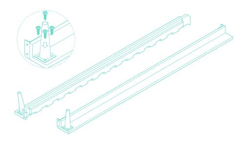
Attach a front leg (**H**) to the corresponding side rail (**C**) by matching the base of the leg up to the existing pilot holes and threading four 16mm phillips screws (**B**) into each hole. Tighten with a screwdriver. Repeat on the other side rail.
