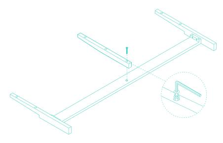
Attach the center headboard post (**F**) to the headboard bar (**G**). Align the existing pilot hole at the base of the center post to the center hole of the headboard bar. Thread a 30mm hex screw (**7**) with one spring washer (**8**) and one flat washer (**9**) through the center pilot hole to secure. Make sure the washer follows the pictured order. Tighten with the small allen wrench (**5**).
