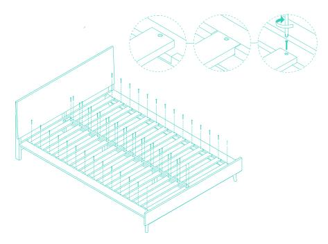
Prop one slat (**D**) into each of the slots on the center beam and side rails. Use a 32 mm phillips screw (**2**) to secure the slats to each side. Continue down the line. Tighten with a screwdriver.
