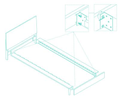
Connect the side rails (C) to the headboard (A) and footboard (B)
