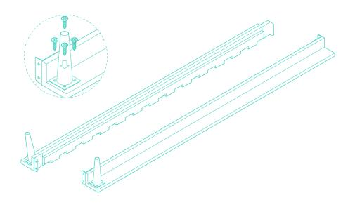
Attach a front leg (**G**) to the corresponding side rail (**C**) by matching the base of the leg up to the existing pilot holes and threading four 16mm phillips screws (**3**) into each hole.
