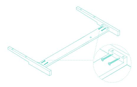
Attach the side headboard posts (**E**) to the headboard bar (**F**). Align the existing pilot holes of the side post to the holes of the headboard bar. Make sure the notch of the side post is facing the front of the support beam – as pictured. Thread two 32mm phillips screws (**2**) into the pilot holes to secure. Tighten with a screwdriver. Repeat on the other side.
